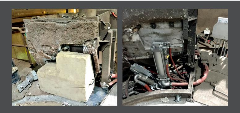
HTT TAPEYETM SYSTEM WITH CAMERA AND HOPPER ON EAF ROOF WITH / WITHOUT COVER
